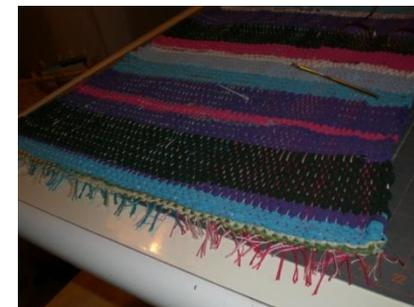
As you can see in the picture above, the weaving is off the loom and the ends of the warp threads are being tied-off.
