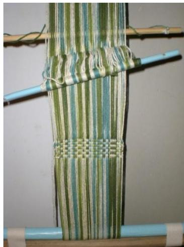
An end string is attached to the alternate shed rod to secure it from falling out of the shed; no need for this precaution on the string heddle. The first 6" is not woven on each end because that section will be braided for the backstrap attachment on each end.
