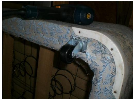
The caster is swivel with ball bearings and is rated for 50 pounds each. I place 6 total casters so that's 300 pound maximum weight.
